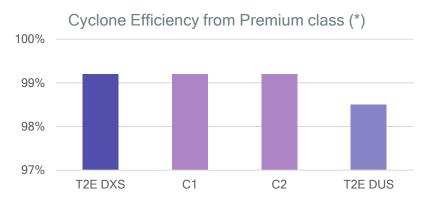
(\*) Whereas: 15,000 m3/h of air at 85oC (30 g/kg AS) with particle size distribution: d50:  $30\mu m$  d85:  $50\mu m$  and d15:  $10\mu m$ , with *AirLock device* and pressure loss of 2,000 Pa.
